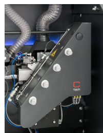
2 motors tiltable End Trim unit
