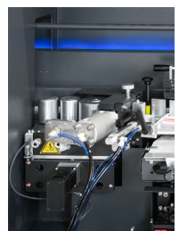
Pressure Rollers station w/ Motorized adjustment
