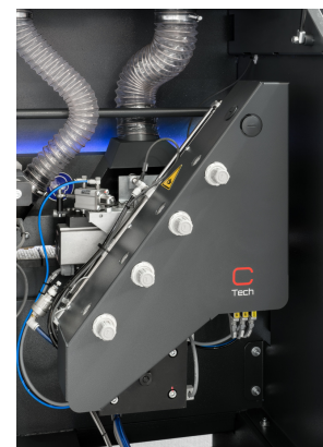
2 motors pneumatic tilting End trim
